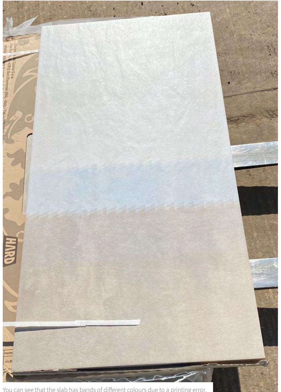
You can see that the slab has bands of different colours due to a printing error.
